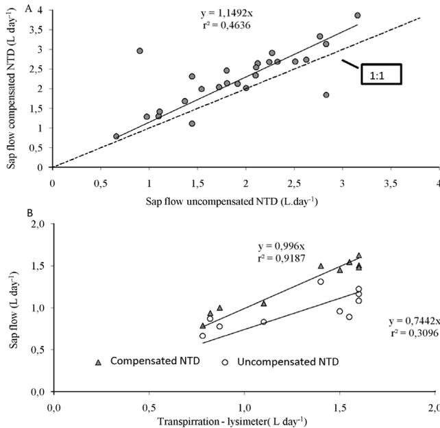
**Figure 7.** Relationship between the average daily sap flow period (FS) for each plant with and without compensation of the natural temperature differences in the stem - NTD (A) and relationship between the lysimeter measured and cumulative daily sap flow with and without NTD compensation (B)
