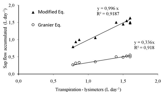
**Figure 6.** Relationship between transpiration measurements made with lysimeter and sap flow accumulated daily by the heat dissipation probe
