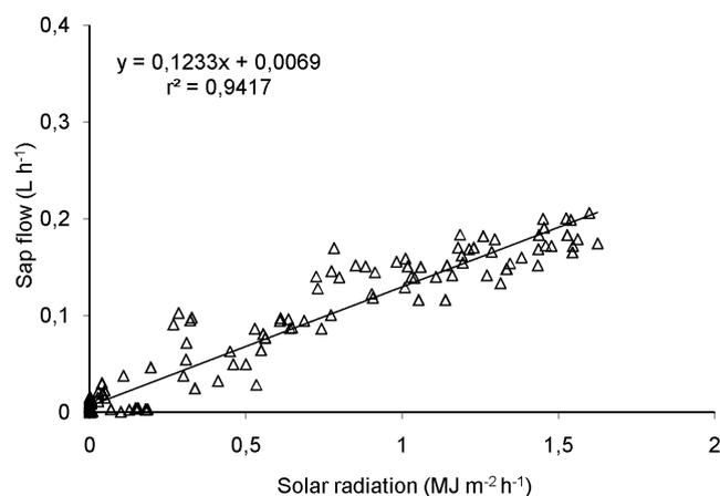
**Figure 5.** Relationship between sap flow by the equation of Granier calibrated to Tabasco pepper and solar radiation as an hourly mean (Piracicaba, São Paulo, July 25 to August 4, 2010)
