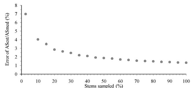
**Figure 8.** Percentage error in the relationship between measured and estimated conductive area ( $AS_{est}/AS_{med}$ ) versus percentage of stems sampled
