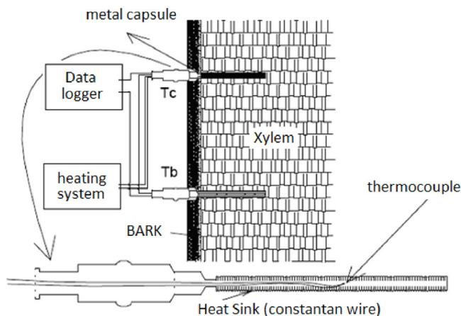
Tc-heated probe; Tb-reference probe
