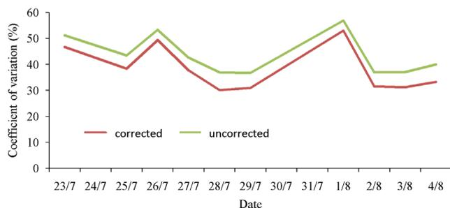
**Figure 9.** Coefficient of variation of daily measurements of sap flow in Tabasco pepper with and without correction of the effect of positioning the probe
